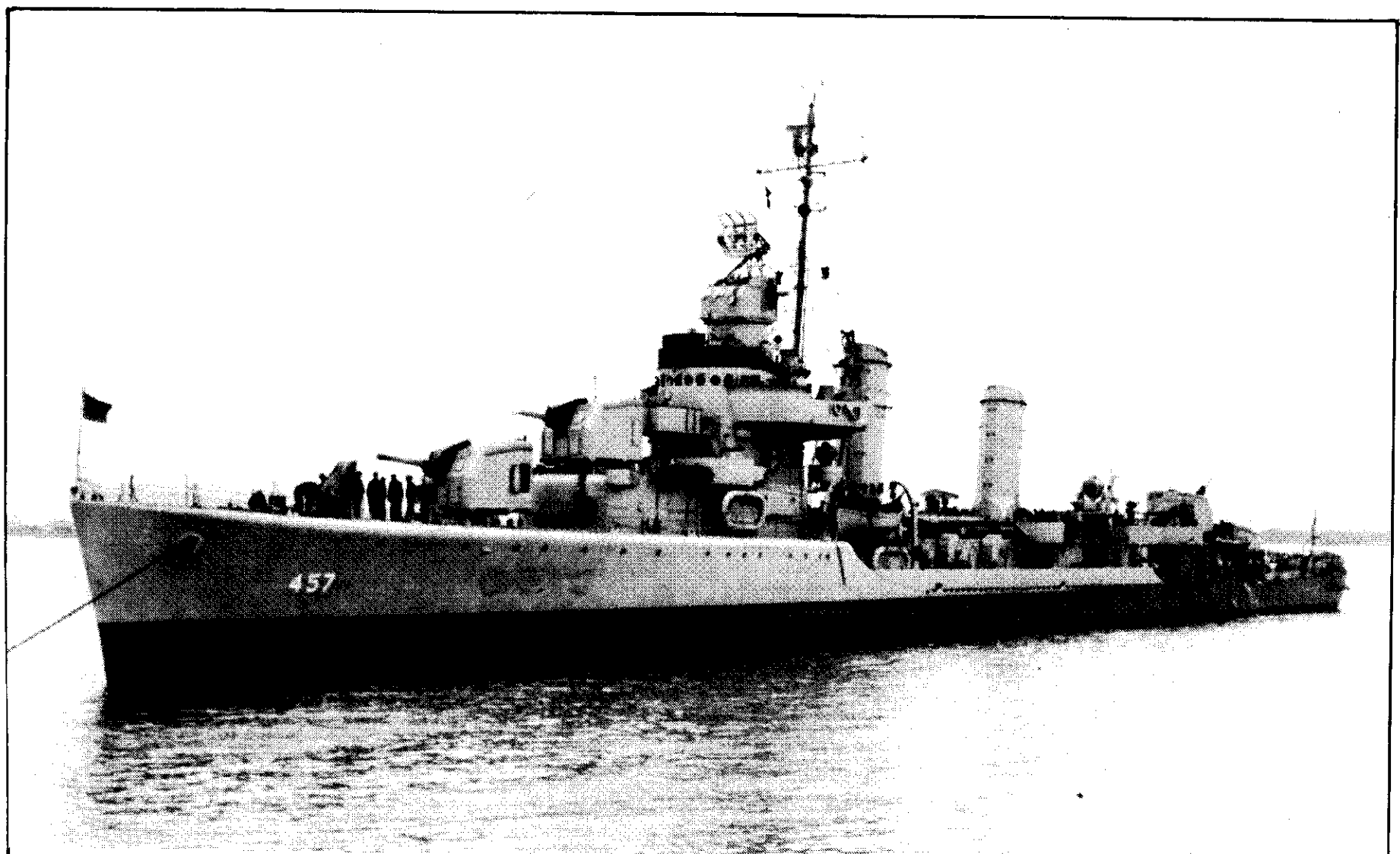
The U.S.S. Emmons (DD-457) (Lt. Comdr. Harold M. Heming, USN) in New York Harbor after her availability at the Navy Yard there from 26 January to 3 February 1943. Note the twin 40-mm. Bofors gun mount on the port side of her after gun platform, just forward of Mount No. 3. The Emmons was armed at this time with seven Oerlikon 20-mm. antiaircraft guns; three forward of the bridge in a bilevel arrangement, two on the bridge wings and two abreast the after funnel. (Official U.S. Navy Photograph.)
